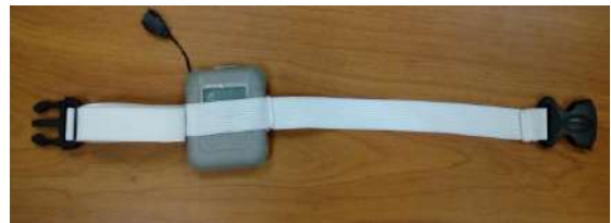
Figure 1: Specifically made and pre-tested neck band to fix the dosimeter.
