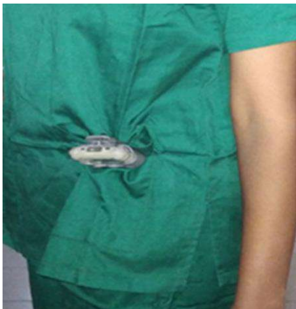
Figure 02: Hp(10) dosimeter positioned under the lead apron
