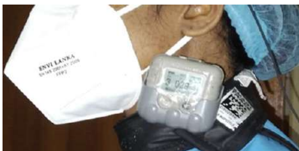
Figure 01: Hp(10) dosimeter positioned above the thyroid collar.
