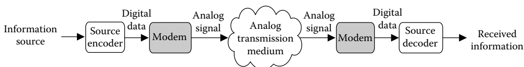
FIGURE 1.3 Generic communication system incorporating a modem.
