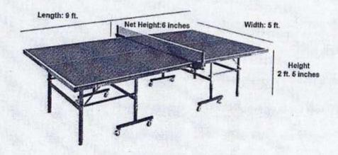
According to ITTF rules of table tennis, the standard table dimension must be 9 feet(length) x 5 feet(width) x 2 feet 5 inches(height) or 2.74m (length) x 1.525m(width) x 76cm(height). While the net need to carry a height of 15.25cm or 6 inches measure from the table surface. This includes either indoor or outdoor tables.
